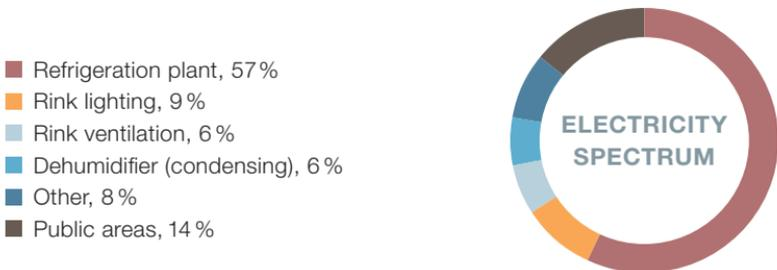
Annual electricity consumption is 960 MWh with mechanical dehumidification (900 MWh without dehumidification).
